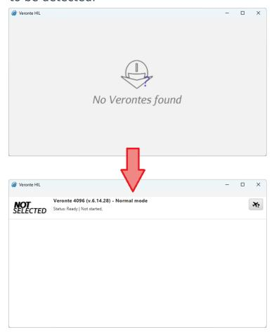
**HIL** detection of connected autopilot
