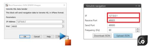
**Simulink Navigation - Data Sender configuration**
